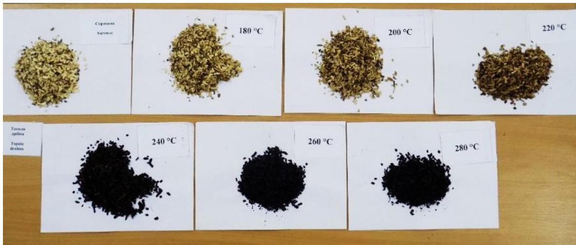
Fig. 2. Visual appearance of poplar biomass before and after torrefaction at different temperatures
