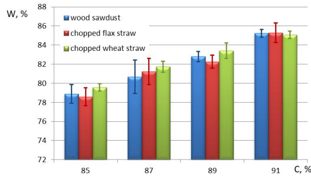
Fig. 2. Histogram of the average moisture content W of the mixtures at sapropel contents C
