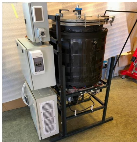
Fig. 4. Laboratory-scale model of microwave-assisted sublimation system developed within the SubliMik project
