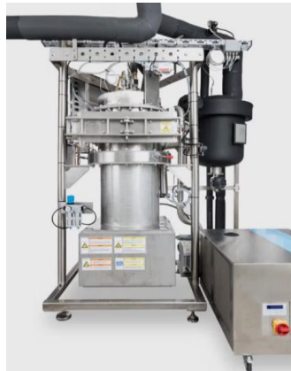
Fig. 1. Technical University of Munich and GEA Group AG prototype of microwave-assisted freeze-drying system for pharmaceutical applications
