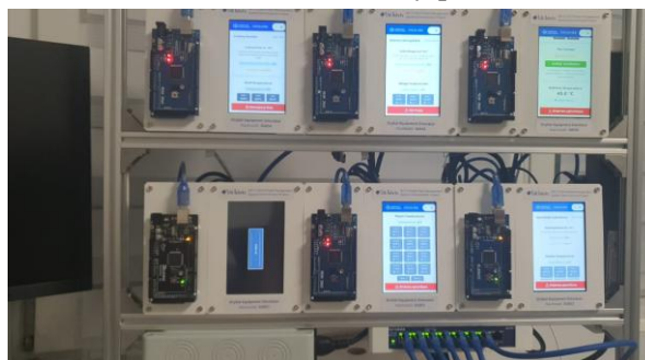
Fig. 3. Distributed laboratory test platform with simulator nodes
