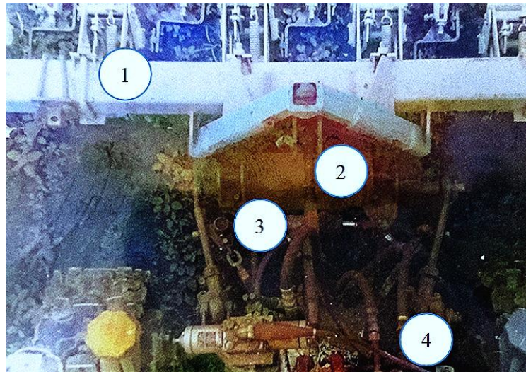
Fig. 3. Controlled tractor hitch mechanism coupled with the USMK-5.4B cultivator: 1 – cultivator frame; 2 – correction device; 3 – hydraulic cylinder; 4 – tractor hitch
