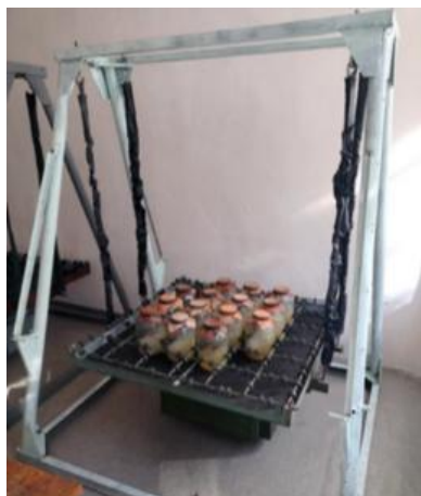
Fig. 1. KPM 36/90 suspended microbiological shaker
