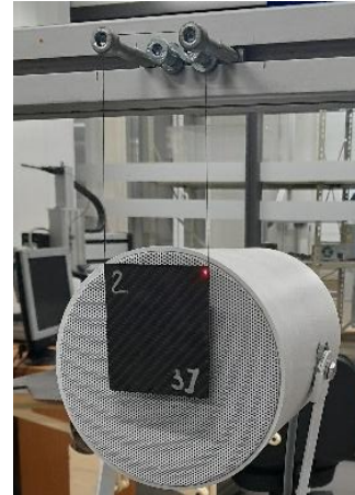
Fig. 3. Specimen with free-free boundary conditions excited by loudspeaker
