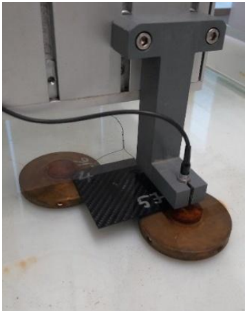
Fig. 2. Ultrasonic scanning of specimen in water
