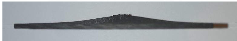
Fig. 6. Curved shape of specimen after impact
