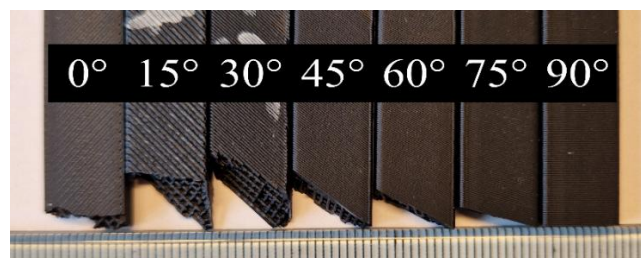
Fig. 3. Fracture behaviour of the specimens at each orientation angle (scale bar: 1 mm)
