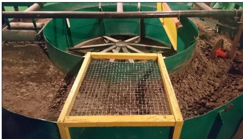
Fig. 6. Photo of the installation for modeling the movement of working bodies of soil tillage machines
