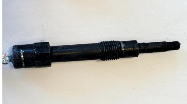
Fig. 2. Modified glow-plug holder with an installed thermocouple for direct temperature measurement inside the combustion chamber
