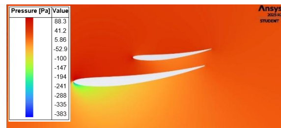
Fig. 11. Pressure contour of open-flap, 2D analysis
