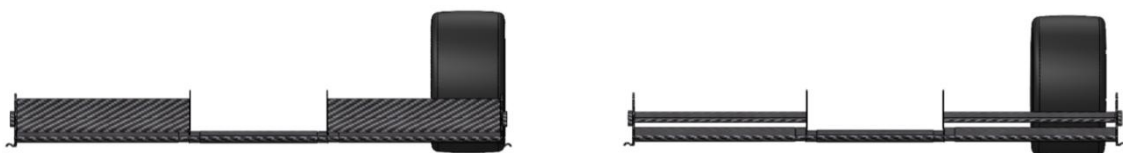
Fig. 1. Front view of the closed-flap front wing Fig. 2. Front view of the opened-flap front wing
