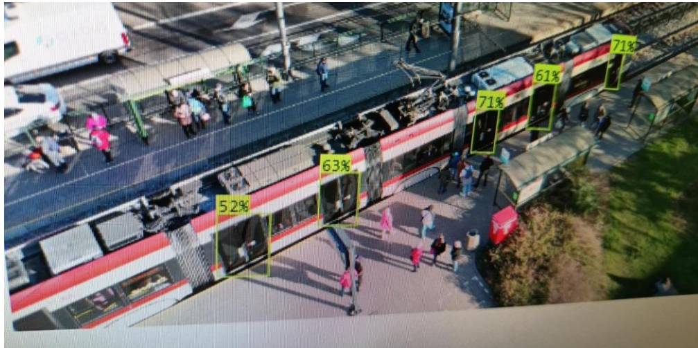
Fig. 1. Example of how the proprietary object classifier works – doors of rail vehicles
