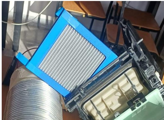
Fig. 4. Cabin filter mounting frame attached to the test stand
