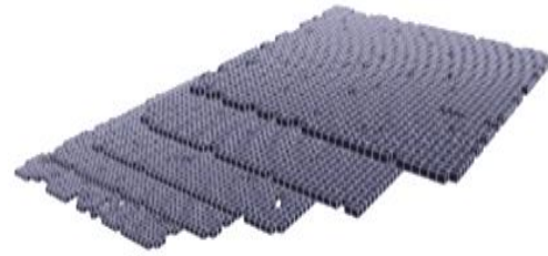
Fig. 2. Stratification of the 3D powder-layer model into voxel sublayers
