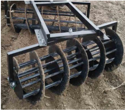
Fig. 2. General view of a harrow with screw-type working bodies: a – machine-tractor unit; b – JINMA 404 E tractor and harrow with screw-type working bodies
