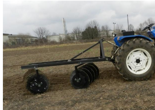
Fig. 2. General view of a harrow with screw-type working bodies: a – machine-tractor unit; b – JINMA 404 E tractor and harrow with screw-type working bodies
