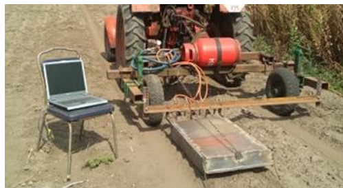
Fig. 2. Laboratory and field studies of the flame cultivation process during post-emergence treatment of table carrot crops
