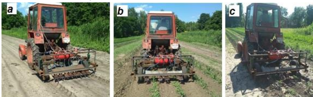
Fig. 6. General views of the units for flame cultivation operations: a – continuous full-width flame cultivation on table carrot crops; b – flame cultivation in rows on maize crops; c – flame cultivation in rows of tomato seedlings
