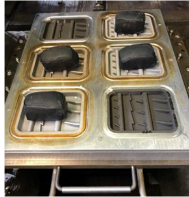
Fig. 3. Mold stored in the machine ready to be pressed with material
