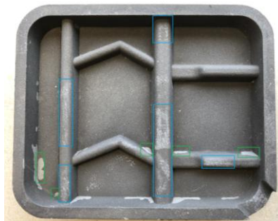
Fig. 4. Prototype with \text{Co}_47\text{Mo}_33\text{Cr}_18\text{Si}_2 coating with summer tread pattern after rubber vulcanization test
