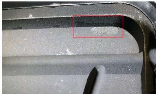
Fig. 5. Stains on vulcanized rubber caused by previous peeling of the coating first vulcanized rubber in summer form coated with \text{Co}_{47}\text{Mo}_{33}\text{Cr}_{18}\text{Si}_2 powder
